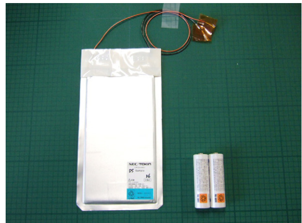
Fig. 2. Lithium-ion pouch cell used for REIMEI.
